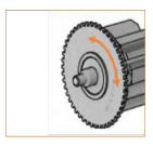
This end of the blind contains either a female or a male pin that can be extended or concealed by turning the wheel. Concealing the pin can help during installation if the fit is tight. If the blind does not reach,
